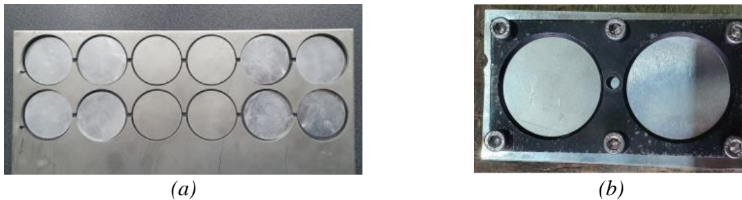
Figure. 1 (a) Final results of 316L SS sheet after water jet cutting; (b) sample support integrated in the AP-plasma deposition method;
