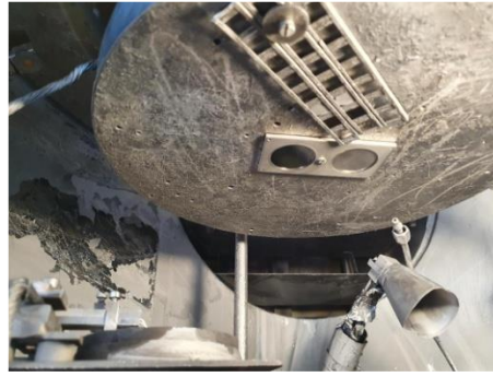
Figure 2(a) Deposition chamber interior of the TVA method with mounted substrates (pre-deposition); (b) Image from CMSII deposition chamber with mounted substrates (post-deposition).
